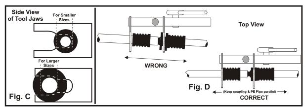
**Caution**: To prevent possible damage to the PE pipe, ensure that the spigot is fully seated in the tool jaw (see *Fig. C*), and that the tool and pipe/coupling is square (see Fig. D) so that the pipe does not drag on the edges of the tool jaw.
