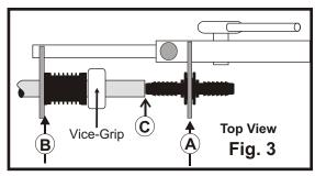
Step 3 Inserting Fitting into Tool
